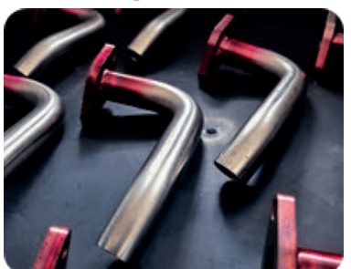
Ressuage Dye penetrant inspection
